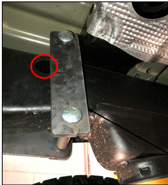
Figure 8: Passenger Side Front Use the hole shown above for fishing Carriage bolt (7) and block (8).
