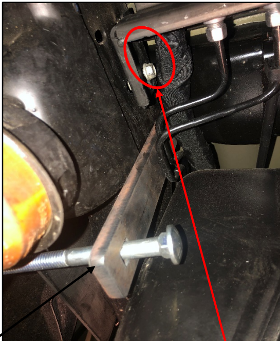
5 Figure 5: Driver Side Front Loosen the 2-brake line support bracket bolts (M8), creating space for mounting block to pass through.
