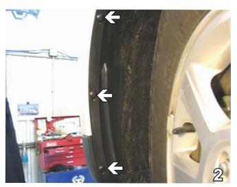
Just forward of the front tire, inside the wheel well, remove three Phillips push pins. Do this to both sides of the vehicle. Set push pins aside to be reinstalled later
