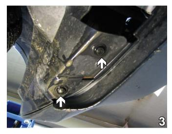
3. Using the 10mm socket, remove two metric bolts from bottom corner of fascia, just forward of front tire. Do this to both sides of the vehicle. Set bolts aside to be reinstalled later.
