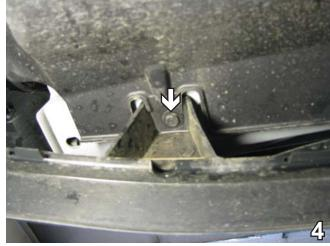
4. Remove three bolts from across the bottom corner of the fascia, using the 10mm socket. Set bolts aside to be reinstalled later.
