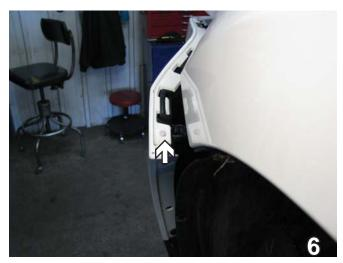
6. Pop out the push pin on the front corner of the fascia. Do this to both sides of the vehicle. Set the push pin aside to reinstall later.
