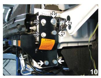
10. Align the baseplate with the seven existing holes in the frame. Insert the existing bolts (gray arrows) with Loctite into the baseplate and tighten. Use 10MM-1.5 x 40MM hex bolts with Loctite and 10MM lock washers in all the holes. In the top two also use a 10MM flat washer. Do this to both sides of the vehicle.
