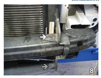
8. Using the flat screw driver, remove push pin from the piece of plastic on the outside of the bumper. Unhook the plastic from the top and the bottom (gray arrow). Do this to both sides of the vehicle. Set aside to be reinstalled later.
