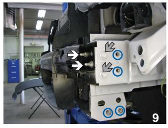
9. Remove the two nuts holding the bumper on with a 13mm socket. Do this on both sides. The bumper core is removed and not reinstalled. Set the nuts and bumper aside to reinstall later. The two bolts on each side (gray arrows) are removed with a 13mm socket and will be used to attach the baseplate. Note: Some vehicles may not have these holes (circled) with threaded inserts, see supplemental options on page 2 for hardware conversion.
