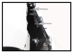
Unclip the fascia on both sides of the vehicle. Using a 10MM socket, reach inside, on the backside of the fascia remove three (3) bolts.
