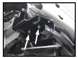
Align the baseplate to allow ample clearance of the air shutter and clamp securely.
