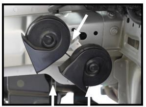
5. On the driver's side, remove the horn using an 8MM socket.
