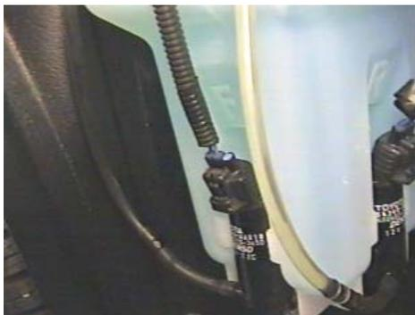
5. Disconnect tubing and plug. Disconnect electrical couplers.
