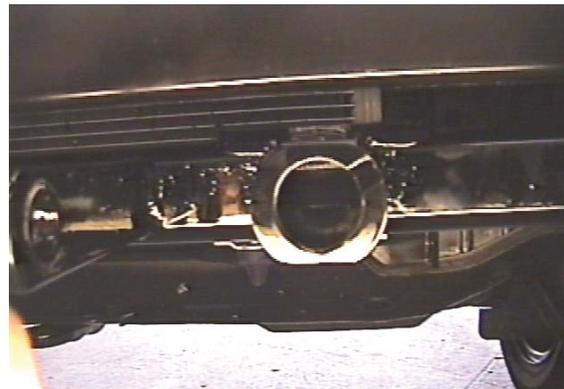
8. Hold baseplate in place. Temporarily clamp baseplate to the bottom side of metal bumper, while holding a 3/4" space between the bottom of metal bumper and cross tube.
