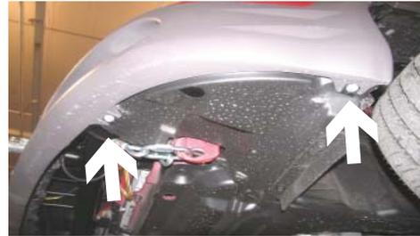
2. Just forward of front tire, on lower corner of fascia, remove two metric bolts with the 10MM socket or a phillips screw driver, both sides.
