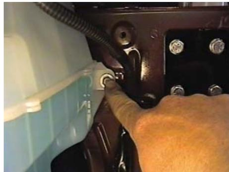
6. Using the 10MM socket, remove the three metric bolts for the windshield washer reservoir and set aside.
