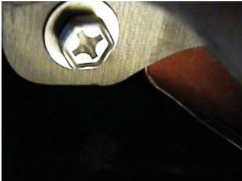
3. Remove metric bolt inside wheel, on fascia's upper corner, with the 10MM socket or phillips screw driver.
