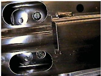
Disconnect wire loom and temperature sensor from the top of metal bumper. Remove two metric bolts from metal bumper openings using the 13MM socket, on both sides.
