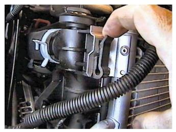
13. Pull clips of radiator to the front to release on both sides. This will allow the radiator to slide up for easier baseplate installation.
