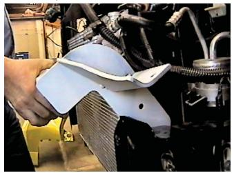
14. Rotate baseplate behind bumper brackets and slide onto frame rails, both sides.
