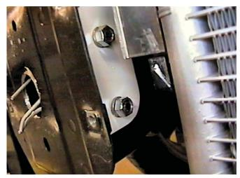
15. Align baseplate with the existing holes on frame, insert bolt plates into cut 1 1/2" hole on bumper bracket, through to the existing holes and baseplate. Tighten 3/8" lock washers and hex nuts, both sides. Be sure and use loctite on all bolts/ hex nuts before tightening. Torque all bolts/ hex nuts according to torque chart in General Instruction sheet.
