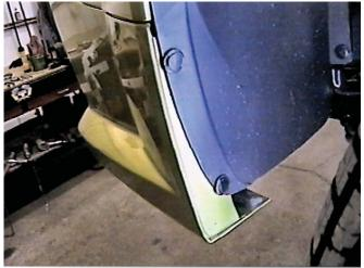
3. Just forward of front tires are four push pins to remove from edge of wheel well and fascia, on both sides.
