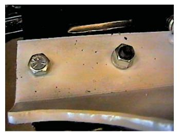
16. Using the baseplate as a template, drill the two holes with the 13/32" drill bit, on both sides. Insert the bolt plate through 1 1/2" hole and into drilled hole, tighten 3/8" lock washer and hex nut, both sides. Be sure and use loctite on all bolts before tightening. Torque all bolts according to torque chart in General Instructions.
