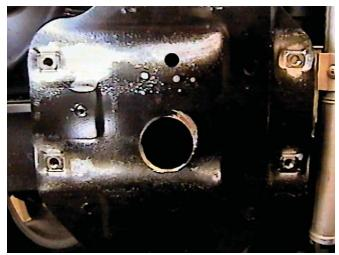
12. Using the 1 1/2" hole saw, cut a hole into bumper bracket to gain access to the inside of frame rail, both sides (passenger's side shown).
