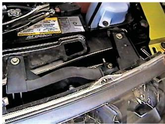
6. Using the 6MM socket, remove two metric bolts from headlight assemblies, pull forward, unplug electrical connections and set aside, on both sides.
