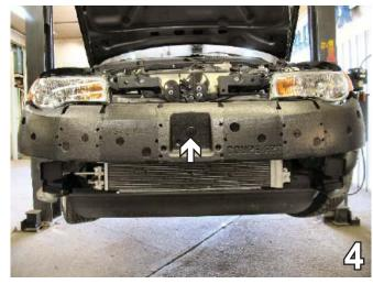
Remove one pushpin from the Styrofoam bumper.
