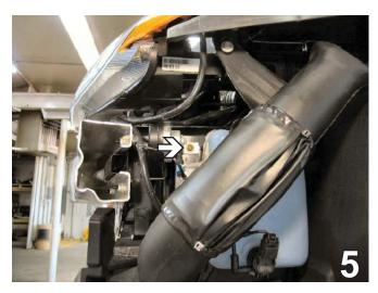
Using a 10MM socket, remove one metric bolt from the horn bracket. Disconnect the horn and bracket. Set all aside to be reinstalled later. Do this to both sides of the vehicle.
