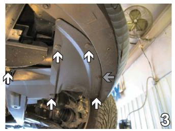
3. Remove six pushpins on the underneath corner of the fascia as indicated by the arrows in the photo. The pushpin indicated by the grey arrow is only on the driver's side of the vehicle. Do this to both sides of the vehicle. Pull fascia corner to the side and release three clips on each side, pull fascia forward. Set the fascia and pushpins carefully aside to be reinstalled later.
