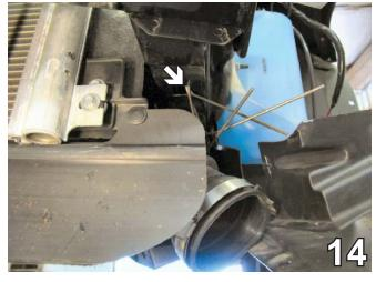
14. Insert the 3/8-16 nut plates up through the opening found underneath the frame and align with the drilled holes. Insert the 3/8-16 x 1 1/2 hex bolts and 3/8" lock washers into the drilled holes, align with nut plate
