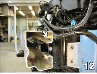
12. Release Christmas tree clip to move electrical cable out of the way for drilling.
