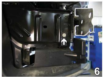
6. Using an 8MM socket, remove one metric bolt from between the metal bumper and the frame rail on the passenger's side and trim away the remaining tab with a utility knife.
