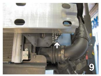
Using the reciprocating saw, cut the webbing under the metal bumper. Cut flush with the bottom of the bumper and the frame rail edge. Do this to both sides of the vehicle.
