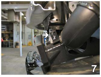
7. On the driver's side, remove one pushpin from between the metal bumper and the frame rail.
