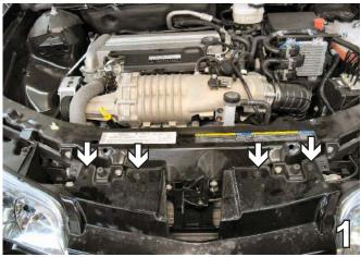
Using a 7MM socket, remove four metric bolts from the top side of the fascia. Set bolts aside to be reinstalled later.
