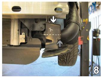
Mark and trim away air dam 1" up from the bottom corner, see the grey arrow in the photo above. Do this to both sides of the vehicle.
