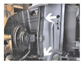
**8.** Pinch clips together on the back of radiator support and pull air dam forward, both sides and set aside.
