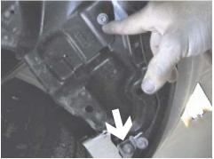
**4.** Forward of front tires, on lower fascia's tabs, are eight metric bolts to remove with the 10MM socket.
