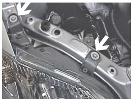
7. Remove four metric bolts from headlight assemblies, pull assembly forward, unplug electrical connection, both sides and set aside.
