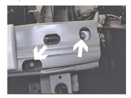
**5.** Using the 12MM socket, remove four metric nuts from metal bumper, pull metal bumper forward and set aside.
