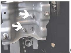
6. Remove two metric bolts from bumper bracket, both sides, pull forward and set aside.
