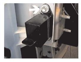
10. Remove top metric bolt from harmonic balancer on passenger's side, insert metric bolt into the three 1/4" flat washers and reinstall to original position.
