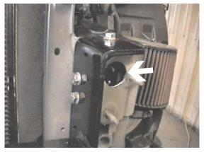
12. Insert 3/8" nut plate into frame end to align with drilled holes, tighten 3/8-16 x 1 1/2" bolt and lock washer with the 9/16" socket, both sides.
