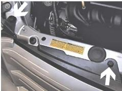
1. Remove the four push pins from the top edge of front grill.
