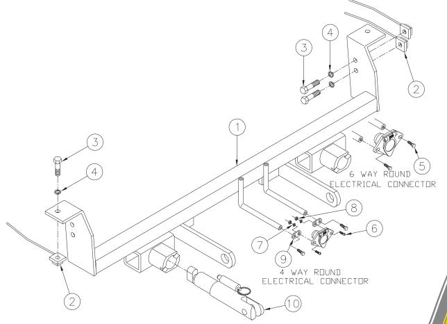
**IMPORTANT:** Use only genuine factory replacement parts on your Base Plate. Do not substitute homemade or nontypical parts. If a bolt is lost or in need of replacement, for your safety and the preservation of your Base Plate, be sure to use a replacement bolt of the same grade (Usually Grade 5, refer to parts list). Repair parts may be ordered through your nearest **Blue Ox** dealer or distributor.
