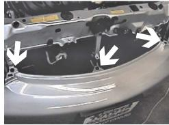
2. Remove two metric bolts from top edge of fascia's tabs with the 10MM socket. Remove one push pin.
