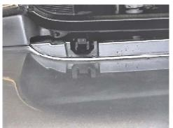
1. Using the flat screw driver, press the six retainer clips in on black plastic cover on top side of fascia, lift to unsnap the back clips on cover and set aside.
