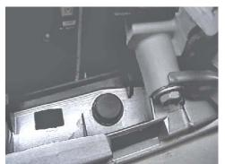
**2.** Just under black plastic piece on the top edge of fascia are three push pins to remove.
