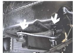
6. Remove two push pins from rubber air dam on the bottom of frame and two from the top of rubber air dam and set aside.
