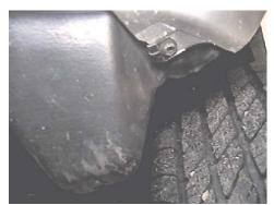
5. Remove the nine metric bolts on the bottom side of fascia using the 10MM socket. Pull fascia forward, unplug electrical components and set fascia aside.
