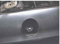
**7.** Using the 14MM socket, remove the four metric bolts from metal bumper, pull forward and set aside.
