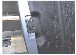
**3.** Just forward of front tire is one metric bolt to remove with the 10MM socket, both sides.
