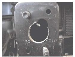
**8.** Drill a 1 1/4" hole in the end of frame rail cap with the 1 1/4" hole saw.
