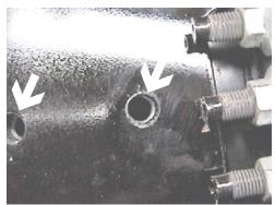
**11.** Using the rubber mallet, align side holes on baseplate (61-6065) with support plate holes (101-6691) as shown in the drawing on the last page and resecure with vise grip. Drill top holes of baseplate with the 13/32" drill bit while maintaining alignment of side holes, both sides.
