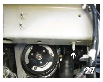
27. On the passenger side on the bottom of the frame, use a pliers to wiggle the stud off.
