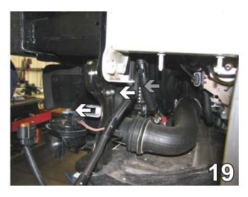
19. On the driver's side, use an 8MM socket to remove the hex nuts holding the horn bracket. Unplug the wire (gray arrow) and set the horn bracket aside to install later.
