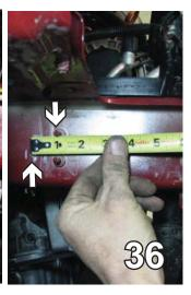
36. On the passenger side, drill a 13/32" hole 1 1/4" up and 3/4" back from the back of the frame end.
