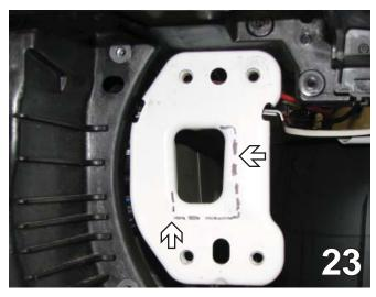
23. On the frame rail end, cut with a reciprocating saw even with the inside of the frame and down. Be sure not to cut into the frame. Do this on both sides. Photo shows driver's side.
