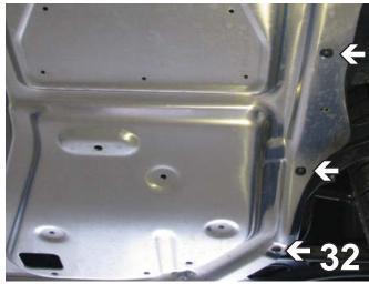
32. If the two bottom holes of step 30 do not line up, it may be necessary to separate the belly pan from fender well plastic using the T-25 Torx to remove the three torx bolts on both sides. Pull wheel well plastic back to ream existing holes.
