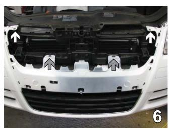
Just behind grille, remove two T-25 Torx bolts at the top (white arrows). And two T-30 Torx bolts in the center (gray arrows). Set bolts aside to reinstall later.
