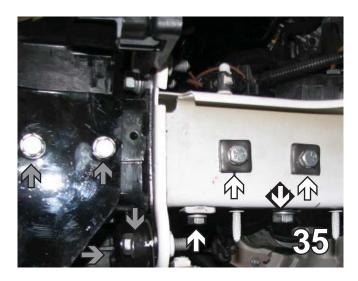
35. Use 3/8-16 nut plates on the inside attached to 3/8-16 x 1 1/2" bolts with Loctite, 3/8" lock washers and 1/4 x 1 x 1" nut plates (white arrows). Four bolts (gray arrows) are 3/8-16 x 1 1/4" with Loctite, 3/8" lock washers and 3/8-16 whiz nuts.
