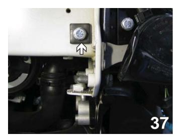
37. Insert nut plates, align with the drilled holes, then tighten 3/8-16 x 1 1/2" hex bolt, 3/8" lock washer, 1/4 x 1 x 1" nut plate into both holes. Be sure 1/4 x 1 x 1" plate is square with the frame to give enough room for the reservoir.
