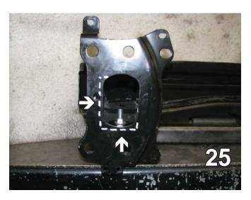
25. On the back side of the bumper with the right side up, cut straight across the opening and straight down following the inside of the extension, then straight across the bottom. Be sure not to cut into the frame. Do this on both sides. Driver's side shown.
