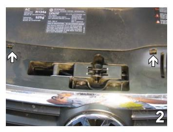
2. Pull back on the two clips in order to remove the plastic. Set plastic aside for later reinstallation.
