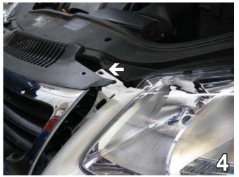
4. Remove the two screws from the bottom of the grille. To remove the grille, lift the clips in the center back to release and lift up over the top edge. Lift the clip in the corner out of the slot. Pull out of the three clips along the side to release.
