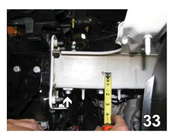
33. Install the 3/8-16 hex bolt, 3/8" lock washer, 1/4 x 1 x 1" nut plate in the front hole on the bottom of the frame and tighten into 3/8-16 nut plate. Do this on both sides.
