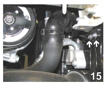
15. On the backside of the frame end just below the frame rail on the passenger side, use an 8MM socket to remove the two hex nuts from the horn bracket. Set aside to reinstall later.
