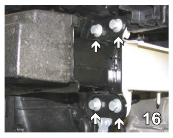
16. Use a 16MM socket to remove the two metric bolts below the headlights and the two on the bottom. Just under the bumper, press the clip down and pull the air dam off. Do this on both sides. Set aside to reinstall later.
