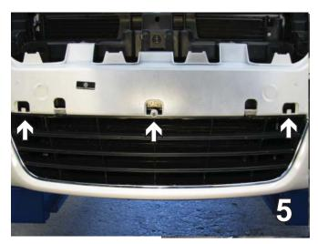
5. Lift and pull out on both sides to slide the three clips out of the notches on the bottom. Some vehicles may have five clips instead of three. Set the grille aside to be reinstalled later.
