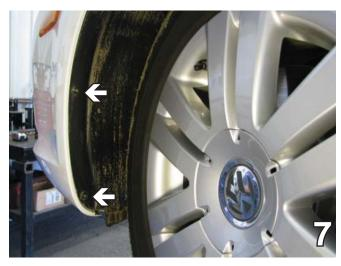
7. Just forward the front tire in the wheel well, remove two T-25 Torx screws. Set screws aside to reinstall later.
