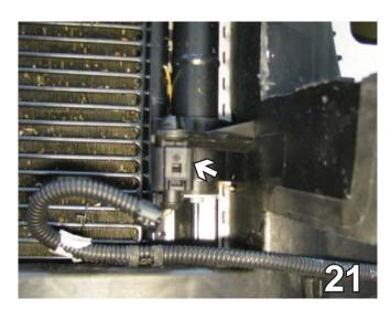
21. Remove the temperature sensor on the driver's side. Turn it around and reinstall so that it is pointing up not down.
