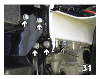
31. Use Loctite and loosely attach all four 3/8-16 x 1 1/4" bolts, 3/8" lock washers and 3/8-16 whiz nuts. Line up the back hole and loosely attach a 1/2-13 hex bolt, 1/2" lock washer, 1/2" flat washer and 61-3799 1/2" nut plate (gray arrow). Do this on both sides. Then tighten up the first four bolts. Reinstall the bracket above the belly pan and the horn brackets on both sides.
