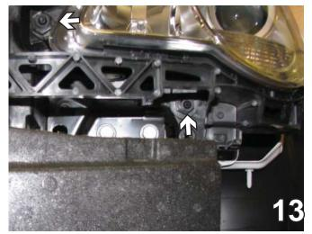
13. Use a T25 Torx to remove one bolt from the side of the headlight and one from the bottom. Do this on both sides and set aside to reinstall later.
