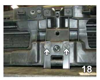
18. In the center of the radiator, use a T-30 Torx to remove the two screws. Set aside for later reinstallation.
