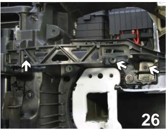
26. Use a T-25 Torx socket to remove the three bolts holding the headlight lower bracket on both sides. Set the bracket and bolts aside to reinstall later.
