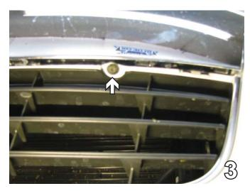
3. Using a T-25 Torx remove the two bolts holding the chrome. Set chrome and bolts aside for later reinstallation.
