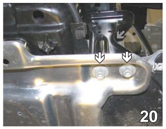
20. Underneath on the belly pan, use a 13MM socket to remove the two hex nuts. Do this on both sides. Take the brace out (gray arrow) in order to remove the bumper. Set all aside to reinstall later. Do this to both sides.
