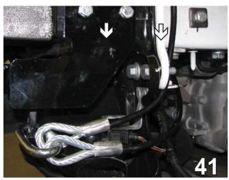
41. On the driver's side, hook the permanent baseplate safety cables around the frame end and under the wires. Do this on both sides.
