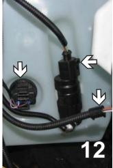
12. Use the 10MM socket to remove the bolt from the top. Disconnect the two electrical connections and the fluid line which should be plugged. Set aside for reinstallation later.
