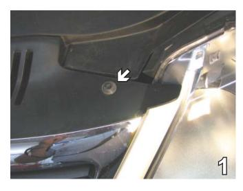
On the top edge of the fascia remove the screw in the corner with a T-25 Torx socket. Do this on both sides and set aside for later reinstallation.
