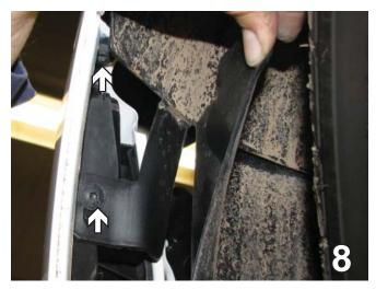
Pull the wheel well cover back and remove two T-25 Torx screws. Set screws aside to reinstall later. Also pull the slide bar back until it clicks to release the clips holding the fascia. Do this on both sides.
