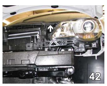
42. Put the headlight brackets and the headlights back in and reconnect.
