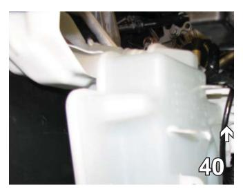
40. On the passenger side, reinstall the washer reservoir. Reconnect the electrical wires and the hoses to the washer reservoir.
