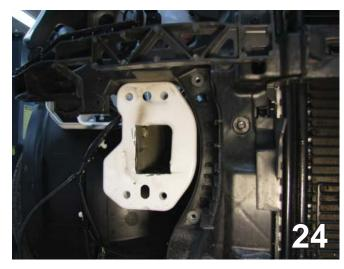
24. Be careful not to cut the nut for the washer reservoir on the inside of the frame on the passenger side.
