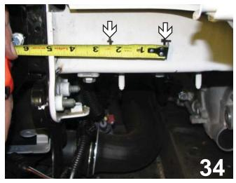
34. On the driver's side, measure up 1 1/4" and over 5" from the back side of the frame end, the next 2 1/2" back, drill first with a 1/4" bit then back it up using a 13/32" drill bit.
