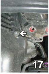
17. Use the T-30 Torx Socket to remove three bolts. Do this on both sides. Set aside for reinstallation later.
