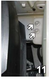
11. Using a 10MM socket, remove one bolt from the front of the washer reservoir and two from the back on the passenger side.
