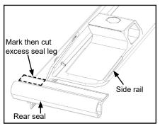
C. Peel paper back, align and adhere seal to end of side rail.
