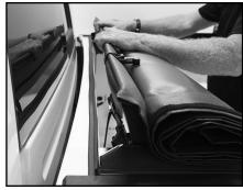
D. Engage springs until thumb wheels are under side rails, then slide bar into place ensuring thumb wheels are seated in notches in side rails.
