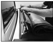
D. Engage springs on thumb wheels and slide thumb wheels under side rail, then slide front bar until thumb wheels are seated in notches in side rails.
