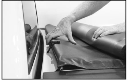
**NOTE:** Ensure alignment tabs are positioned perpendicular to cover and press against bulkhead.
