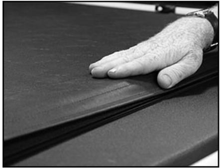
E. For additional protection, manual Slide Lock are located under rear bar on passenger side. Push Slide Lock to engage; pull to disengage.
